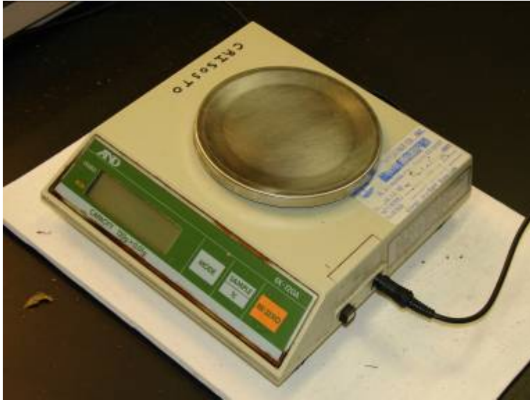
Picture 2. Balance, comparable to Denver Instruments Model MXX-212 with A capacity of 210g, readability of 0.01g, tarring range of 0-210 g If purchased from Fisher Scientific includes operations manual and power supply and calibration weight, cat. No. 01-915-02 ($315.40).
