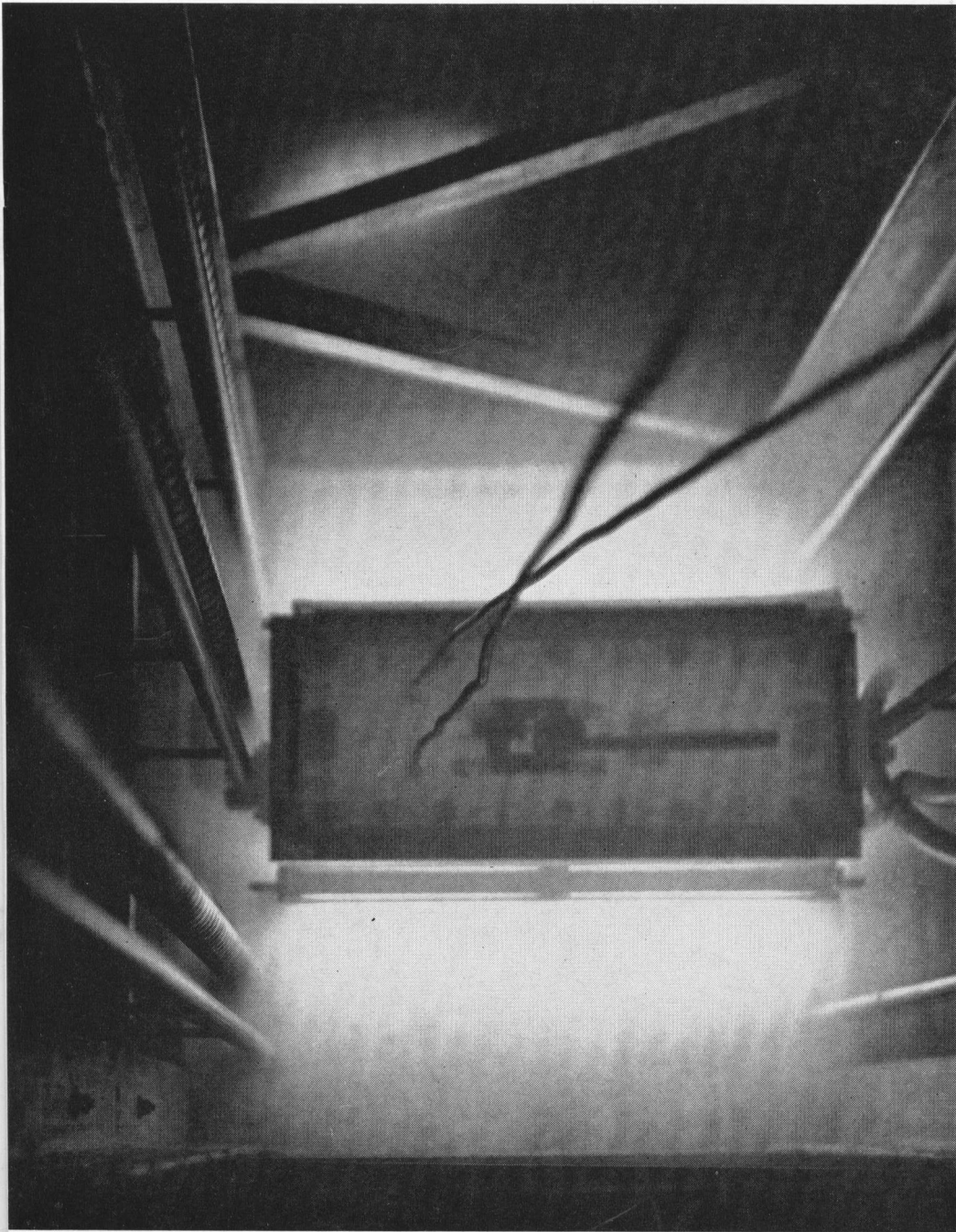
The center irradiation chamber is approaching the radiation field and is seen in the eerie blue light emitted by the radioactive Cobalt-60. Air lines can be seen emerging from the top of the chamber and refrigerant lines on the side.
