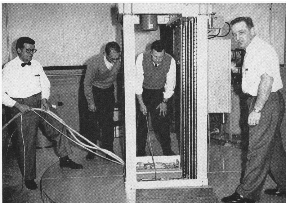
Above—in order to determine the strength and uniformity of the irradiation field, vials containing a chemical dosimeter are arranged as shown above, and lowered in the irradiation chamber.
