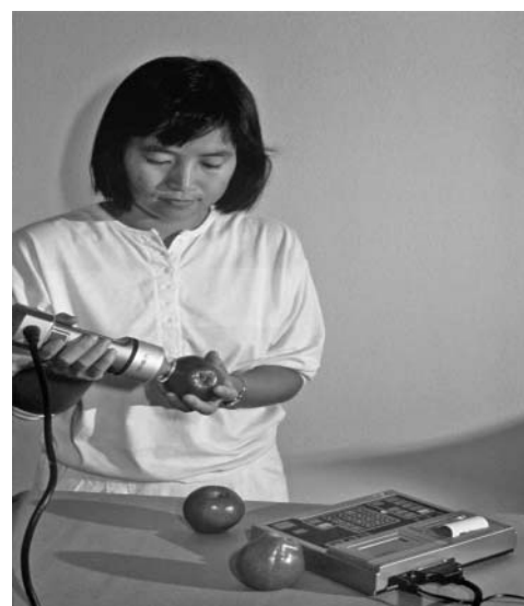
Figure 2 Measuring external color of apples using a Minolta colorimeter.
