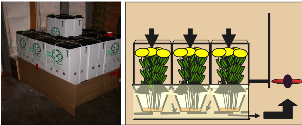
Precooling Procona boxes on a conventional horizontal pre-cooler is achieved by directing the airflow down through the boxes using an adapter plenum, and a fiberboard or fabric sleeve around the base of the boxes.
