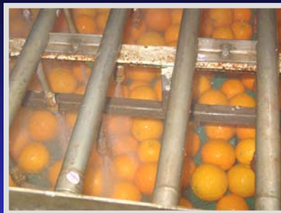
Chlorination on a brush bed (non-re-circulating)
