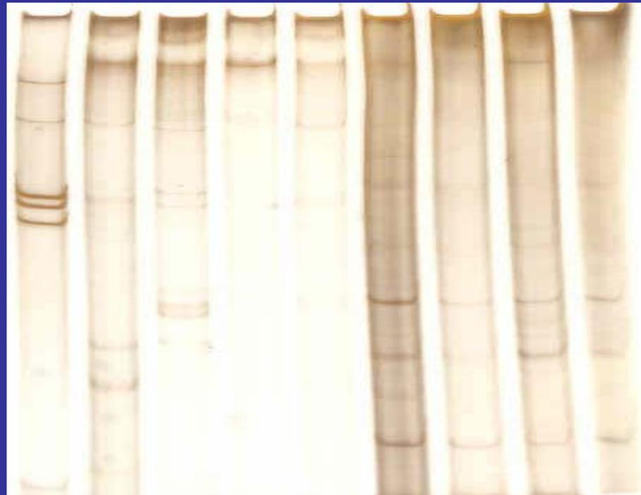
**dsRNAs electrophoresed through 6% polyacrylamide gel and stained with silver nitrate**
