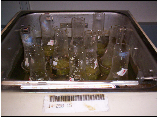
Figure 3.5. Extraction setup for enzymatic pectin extraction of watermelon rind.
