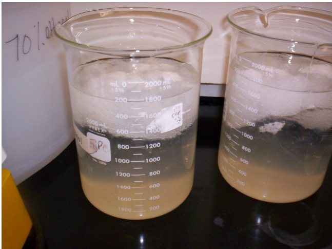
Figure 3.4. Acid extracted watermelon pectin after overnight precipitation.
