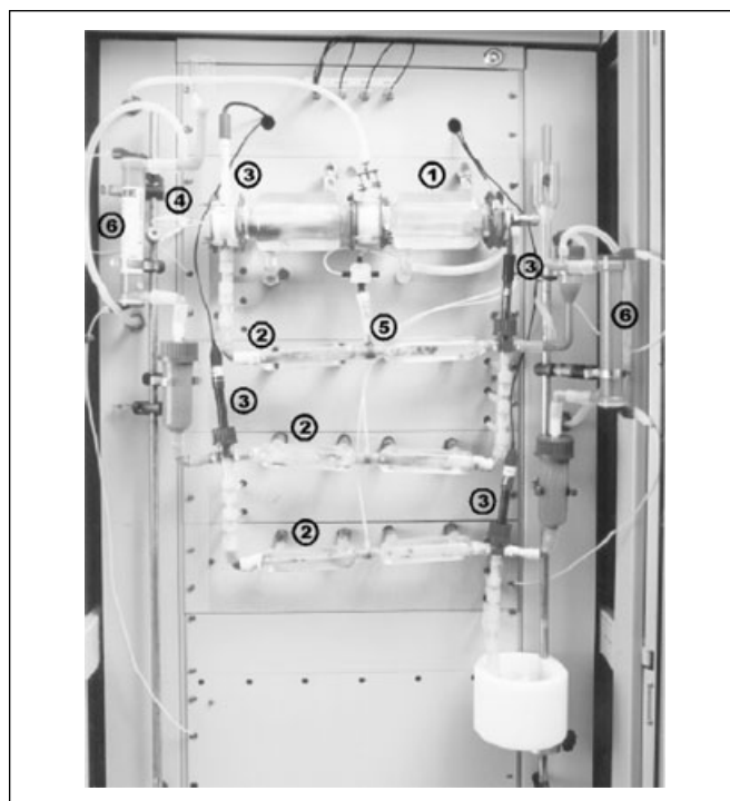
Figure 7 – TNO intestinal model (TIM): (1) gastric compartment; (2) small intestine; (3) pH electrodes; (4) secretion of lipases and pepsin; (5) secretion of pancreatic juice and bile; and (6) hollow fiber membranes simulating the absorption of digested products (Krul 2003).
