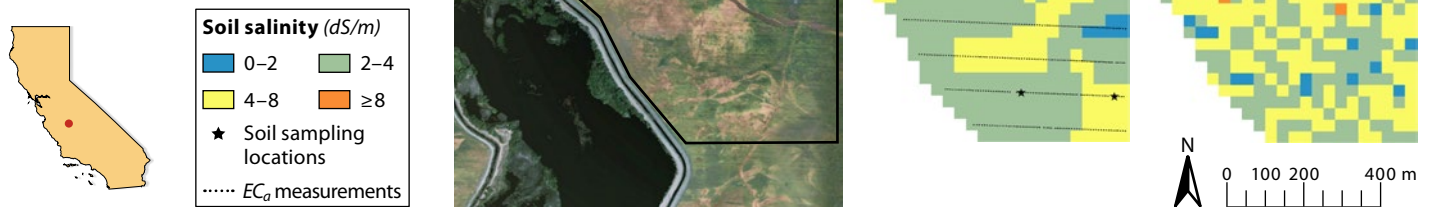
Fig. 4. Example of inaccuracy of remote-sensing estimations in a heterogeneous field with lower salinity values: (A) National Aerial Imagery Program imagery at a test site in Stratford (Kings County) on July 8, 2003; (B) ground-truth root zone (0 to 4 feet) salinity measured by Scudiero et al. (2014) through apparent electrical conductivity ( EC_a ) measurements and soil sampling; and (C) remote-sensing salinity estimations.
