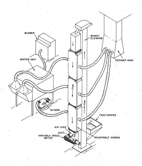
Figure 1. An experimental rice dryer installed in Food Engineering Laboratory, UC Davis.
