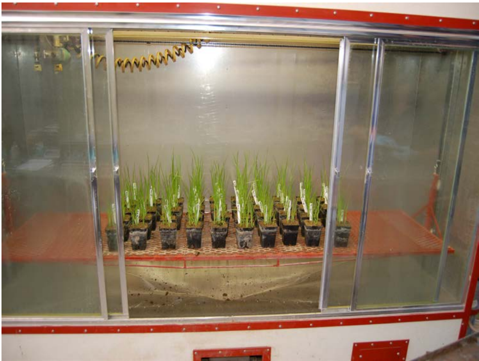
Figure 11. View of plants ready for application in the cabinet track sprayer.
