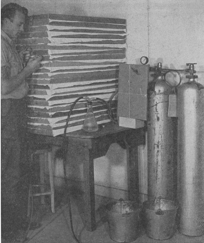
Fig. 17.—Equipment for mixing ether and carbon dioxide and injecting mixture into egg boxes.
