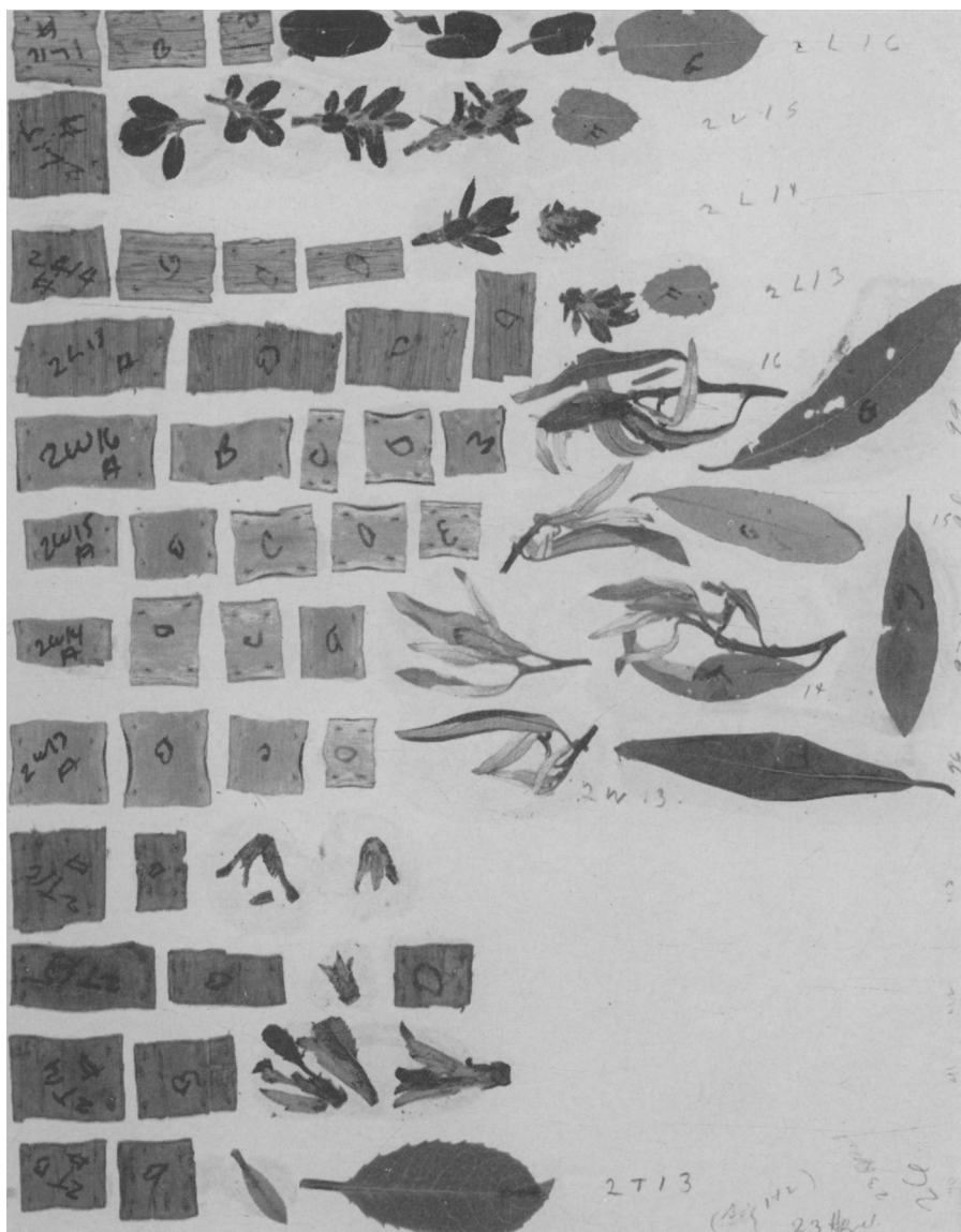
Fig. 1. Samples of bark, stems, and leaves of toyon, arroyo willow, and live oak cemented to a sheet of paper and ready to be placed, face down, on the X-ray film.
