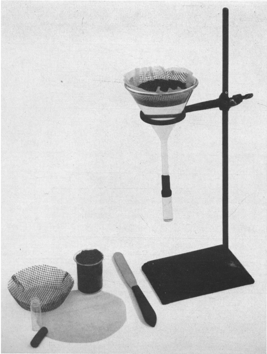
Fig. 2. Type of "Baermann" funnel used to obtain active citrus nematode larvae from soil. A small vial containing water is slipped over the stem of the funnel and secured with a piece of rubber tubing. Then the funnel is nearly filled with tap water. The soil sample is passed through a \frac{1}{8} -inch mesh sieve, then 50 cc of the soil is placed in a wire basket which is lined with tissue paper. The basket of soil is gently placed in the top of the funnel and water is added as needed to maintain the level of the water even with the surface of the soil. After 48 hours at a temperature of 70° to 75° F the vial is removed and the nematodes counted.
