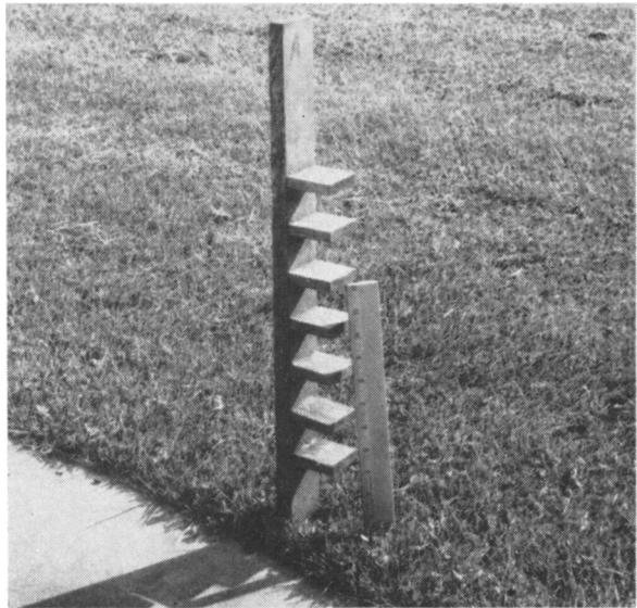
Fig. 4. Varied-level stake used to investigate larval preference of water depth and substrate position in different microhabitats of rice fields.
