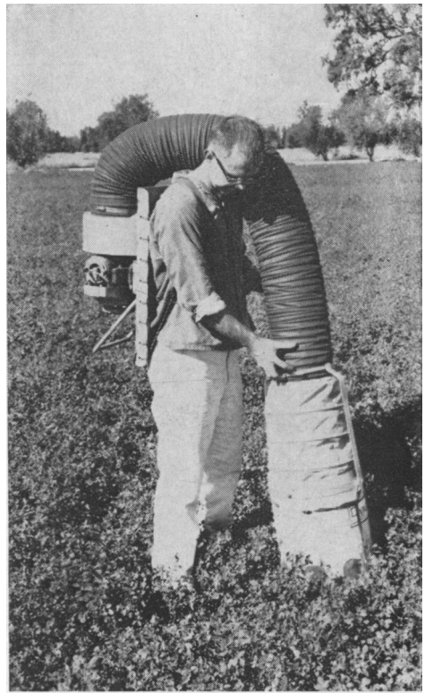
Fig. 1. Back-pack model vacuum machine. The pick-up head has an area of 1 square foot.
