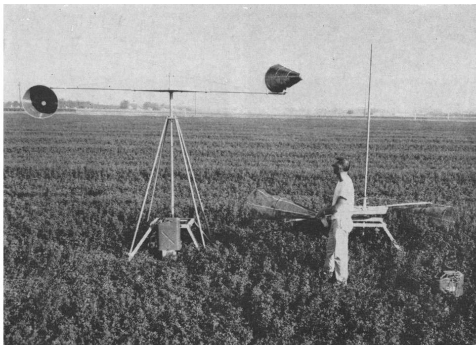
Fig. 2. Rotary net machines used to capture flying alfalfa seed chalcids, shown in a host area with the boom in the high position at the left and in the low position at the right.
