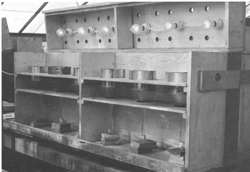
Figure 5. Open Berlese funnel cabinet showing six extraction units.
