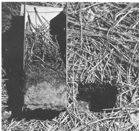
Figure 4. Six-inch coring tool opened to expose soil sample; coring site at right.
