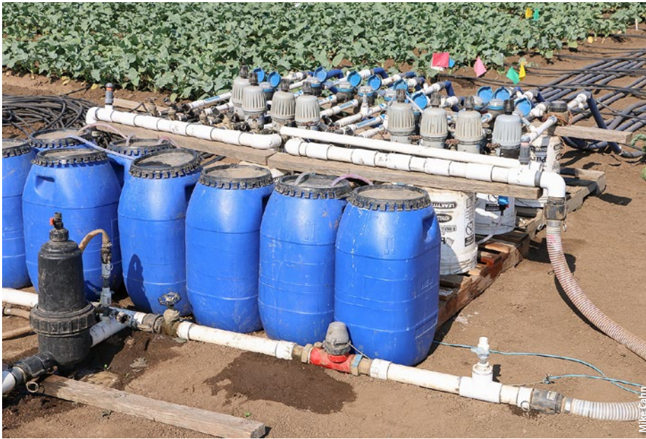
An injection system generated irrigation water with \text{NO}_3\text{-N} concentrations of 12, 25 and 45 mg/L.
