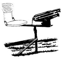
Be careful when cocking the thrower arm or placing a target on it. It can deliver a very powerful blow if released. *Never* release the thrower arm when anything is in its path. It could cause severe injury. Always leave the thrower arm uncocked when the trap is not being used or is unattended. Let's spread out along the firing line and try throwing a target or two.
