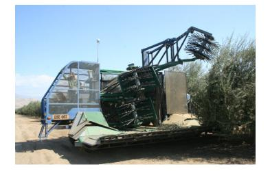
Fig. 1. 2008 version of the canopy contact head olive harvester originally modified from wine grape harvesters in 1996. This harvester can be used as one of a pair, or as a single that does both sides of the tree. The head is mounted on a catch frame that conveys the fruit back to a field bin.
