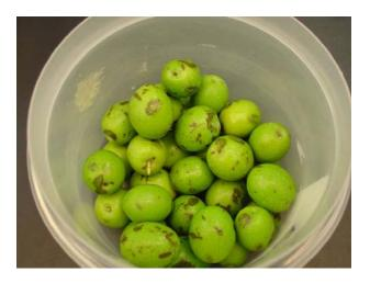
Fig. 2. Bruising and cutting damage produced by Early version of the the canopy contact head mechanical olive harvester in 'Manzanillo' olives destined for California black ripe olive processing.
