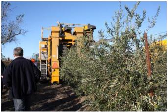
Fig 3. Typical super high density olive oil orchard and straddle harvester.
