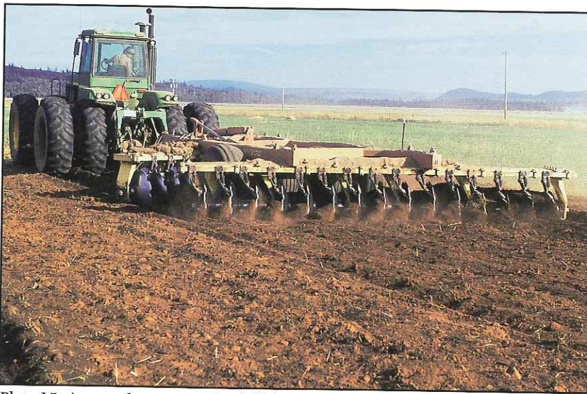
Plate 15. A second pass over the field with the tandem disk at a 45° to 90° angle to the first disking assures more complete incorporation of the ash.
