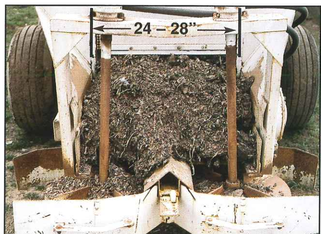
Plate 6. A wide opening in the spreader—24 to 28 inches (61 to 71 cm) wide, as shown here—allows ash to feed properly onto the spinners for uniform distribution in the field.
