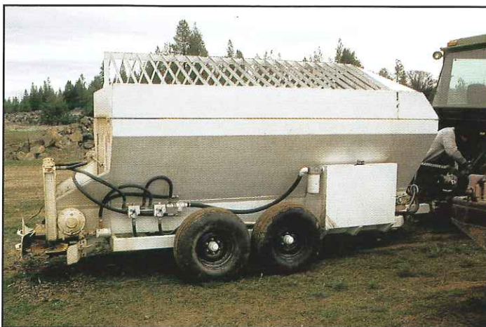
Plate 5. A spreader equipped with a grate or screen on the top can be used to remove large particles from the ash.
