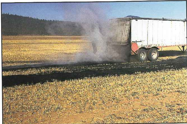
Plate 9. A truck with a moving floor unloads ash in strips in a field.
