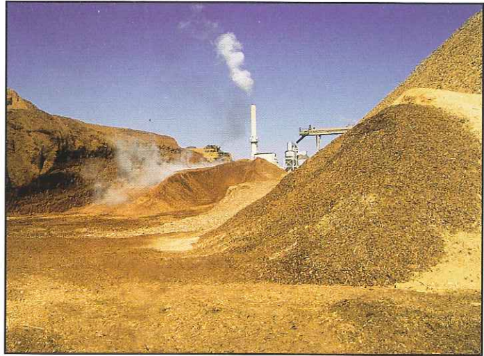
Plate 2. Large piles of wood chips are mixed together before being burned in the power plant in the background.
