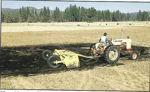
Plate 13. A grader, scraper (shown here), blade, or landplane traveling perpendicular to the windrows can be used to spread the ash uniformly in the field.
