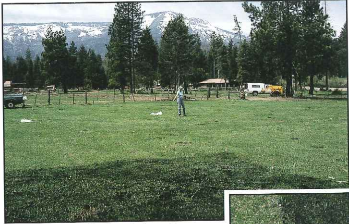
Plate 8. Ash applied on irrigated pasture at 16 dry tons per acre (36 Mg/ha). The inset shows a close up of no ash, left, and ash applied at 16 dry tons per acre, right.
