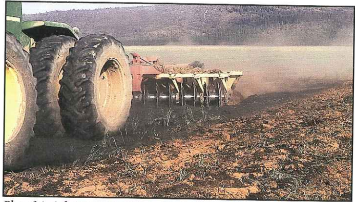
Plate 14. Ash is incorporated effectively using a large tandem or double disk with disks 18 to 24 inches (45.5 to 61 cm) in diameter.
