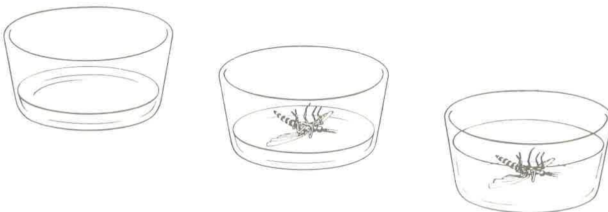
Three steps in embedding an insect in plastic: 1) pour layer of catalyzed plastic into glass mold to harden; 2) place insect in center of hardened layer; 3) pour another layer, covering the insect.
