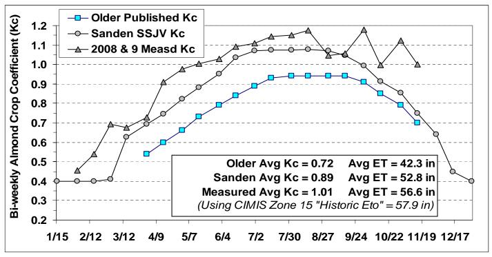
These curves compare the older published Kc curve (39 to 42 inches/year ET) for mature almonds on micro irrigation to Kc numbers developed by Blake Sanden in Kern County through irrigation demonstration monitoring and the 2 year average of a current large-scale field trial. The middle curve is recommended and is used for the next table.
