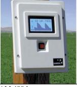
AM 400 logger can accept 6 Watermarks and Temp sensor, \$389
