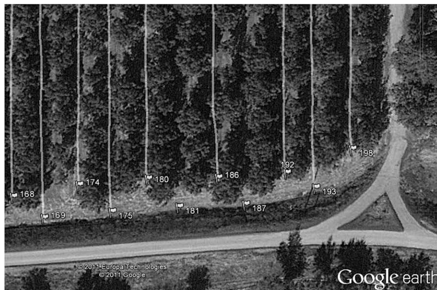
Fig. 3. Geo-referencing information displayed using Google Earth (Google, Mountain View, CA). Flags represent the mobile platform antenna location at point of full sun reading. White lines indicate paths of travel. Image Courtesy of Google and the U.S. Geological Survey (31 May 2007).
