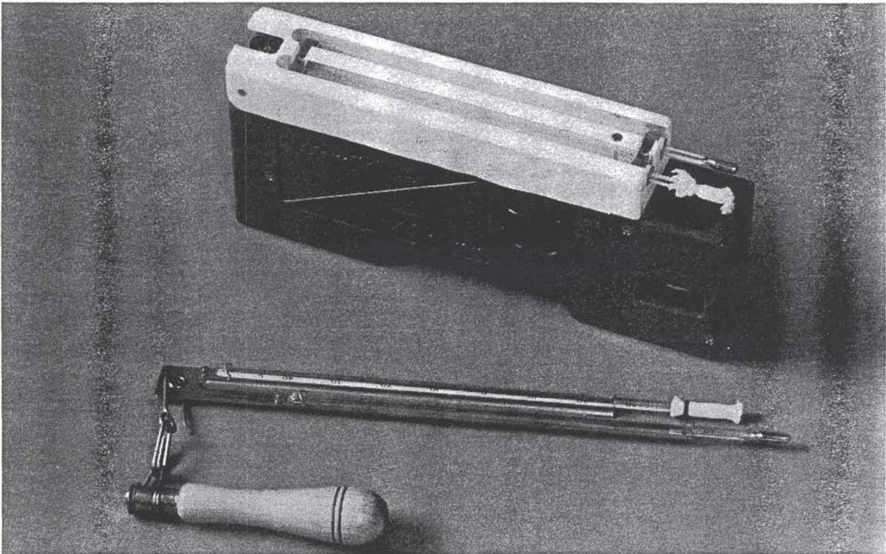
Aspirated (*upper*) and sling (*lower*) psychrometers are used to determine humidity by measuring dry-bulb and wet-bulb temperatures. The cotton wick on a wet-bulb thermometer is wetted with distilled or deionized water, and it is
