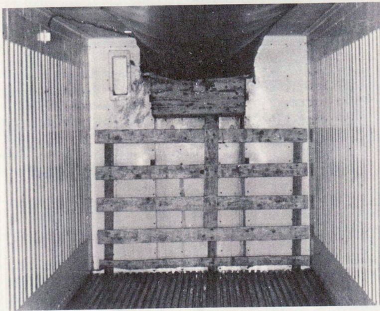
Figure 7.--Bulkhead without false walls, and vertical and horizontal wood strip added to prevent air blockage.
