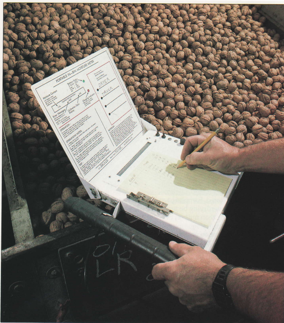
Dryer operator takes moisture reading on full walnut bin using hand held meter. (Moisture readings are displayed as a digital readout, not shown in picture).
