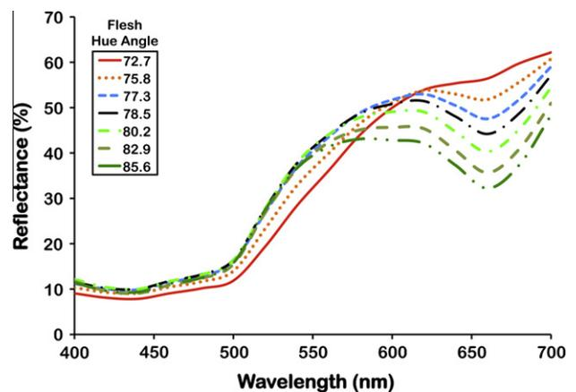
Fig. 4. Plot showing the change in the mean diffuse reflectance spectra of the skin for subsets of peaches with similar flesh hue angles (in degrees).
