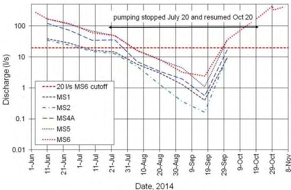
Figure 4—Discharge measurements along the Upper Mattole mainstem in 2014. Pumping cessation period (July 20 through October 20) is noted. Sites are numbered from upstream to downstream order.
