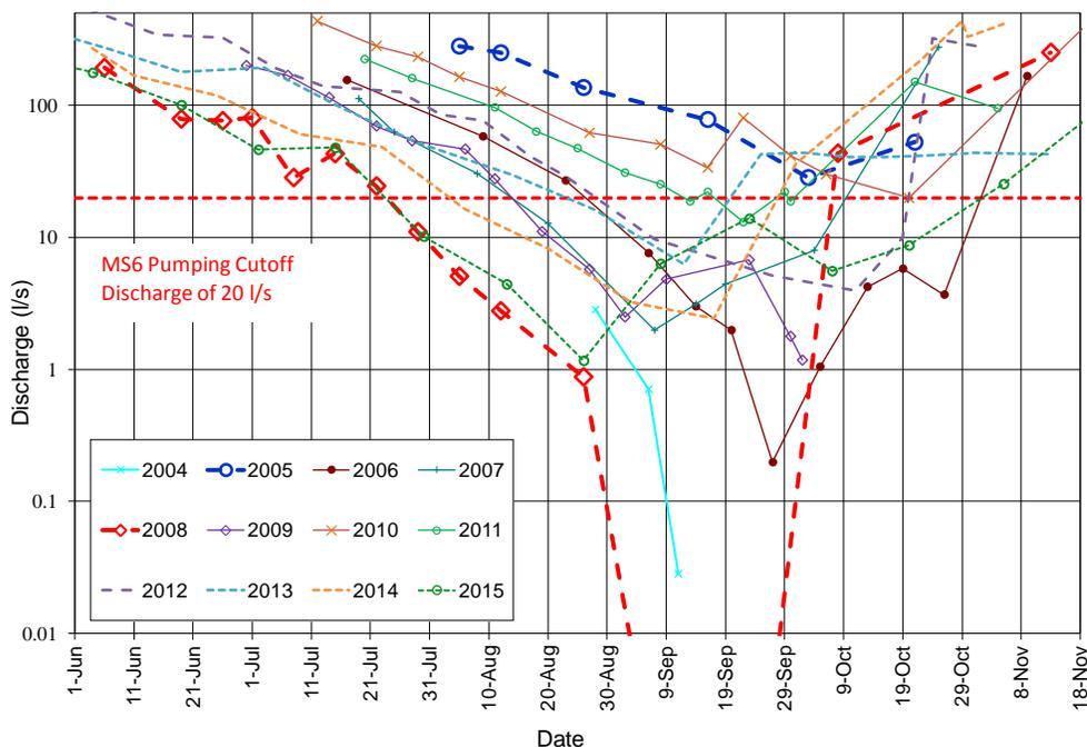
Figure 3—Discharge measurements at MS6, 2004-15 (all dates adjusted to 2016 for plotting). The discharge threshold for cessation of pumping (forbearance) for MS6 (20 l/s, or 0.7 cfs) is also shown. The two heaviest lines indicate flows during 2008 (driest year, dashed red line) and 2005 (wettest year, dashed blue line).
