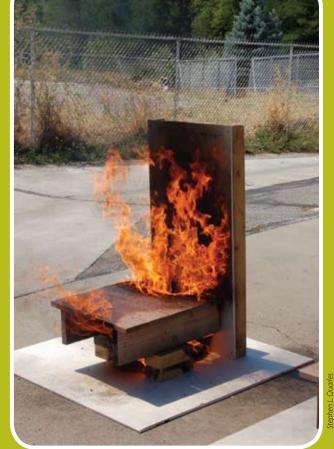
The decking being tested here doesn't comply to Chapter 7A provisions.
