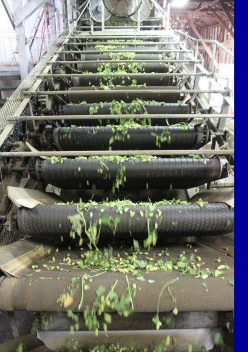
Cones separated on multiple slanted conveyor belts
