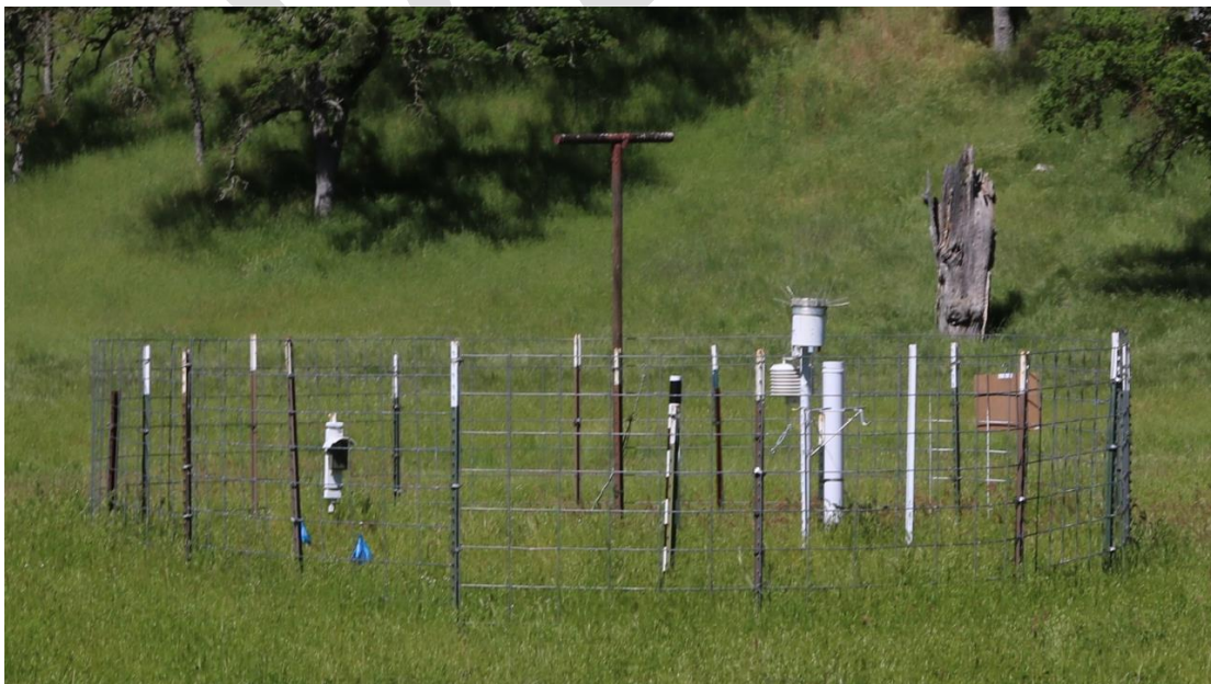
Figure 2. Weather Station Set-up. Each weather station had a 6" tipping bucket rain gauge with a solar shield for the temperature sensor, a non-recording 45" tall, 4" diameter rain gauge and a timelapse camera inside enclosure #4. The bird perch helped reduce birds perching on the rain gauge.
