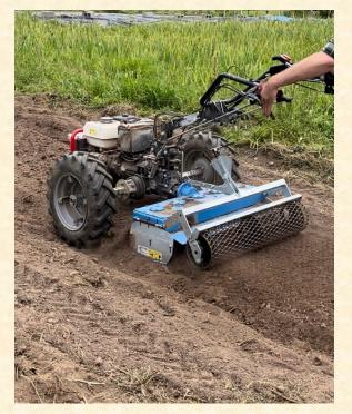
A BCS used for bed prep after tillage on a smallscale farm
