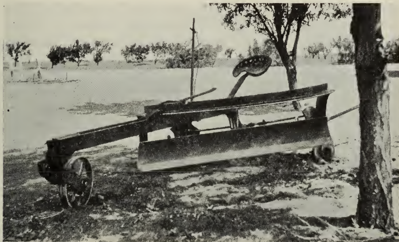
Fig. 39.—A type of grader in common use for constructing broad-base terraces. These are made in sizes suitable for team or tractor operation.
