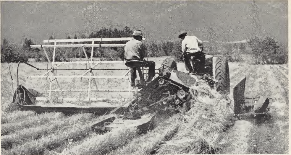
Fig. 5—Binding, shocking to cure and threshing with a mobile machine is the most widely used grass seed harvesting method. The shattered seed on the left of the machine sifts into the metal pan shown dragging beneath and extending to the rear of the binder. Shattered seed from the right side of the machine slides into the tray beneath the bundle carrier. Note short pieces of hose fastened to reel slats. These are centered on the rows and help to keep the cutter-bar free. (Union Pacific Railroad photo.)
