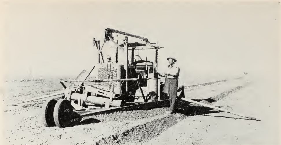
Fig. 6.—Checking attachment for tractor. This machine builds the borders and levels the ground between them in one operation. Machine is equipped with leveling gauge.
