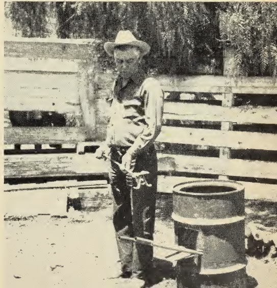
A branding-iron stove, made from an old oil drum, is inexpensive and efficient.
