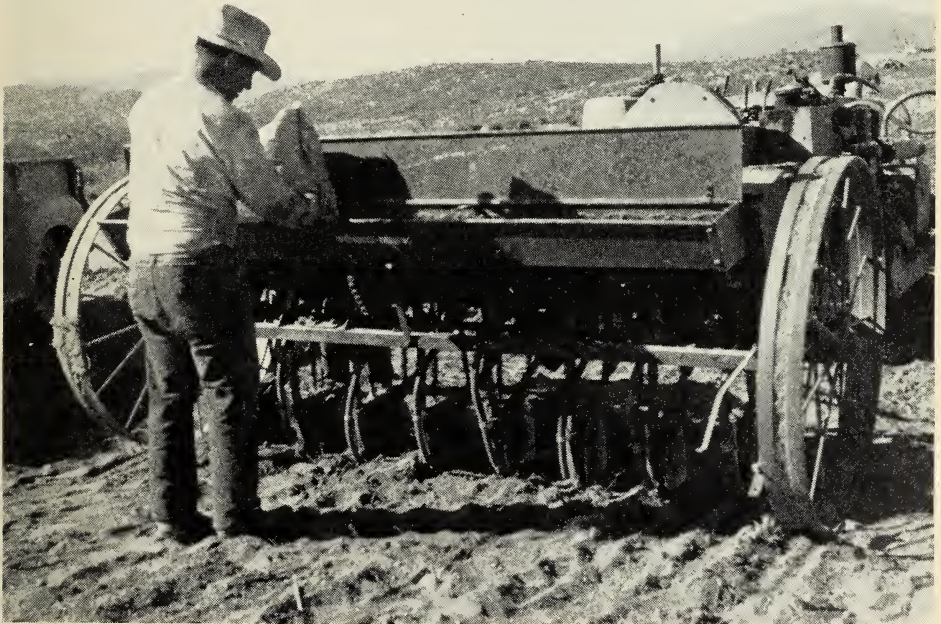
This grain drill was used for placement of seed and fertilizer on a ranch in San Diego County. (Photo by Charles F. Walker)
