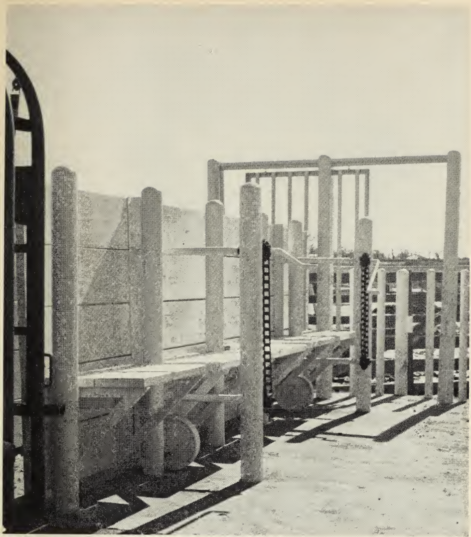
Side view of an adjustable, movable branding chute. Width can vary from 16 to 31 inches. Detail shows hand crank chain and sprocket for adjusting chute.
