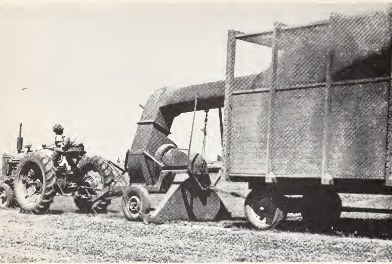
Fig. 35. Left: vacuuming seed. Below: unloading vacuumed seed and trash from seed-tight van with automatic cable-pulley rig. Seed will be recovered with a stationary thresher.
