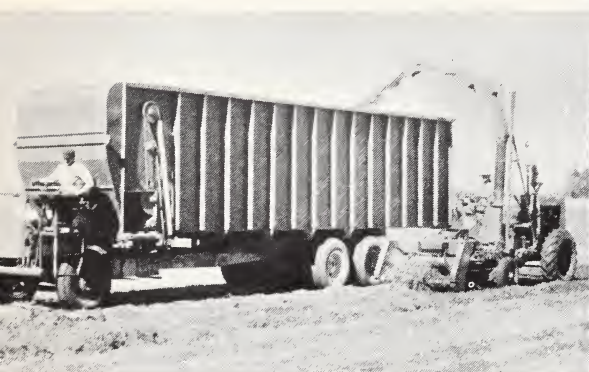
Fig. 16. Spring cleanup with self-unloading van for hauling forage or green feed.
