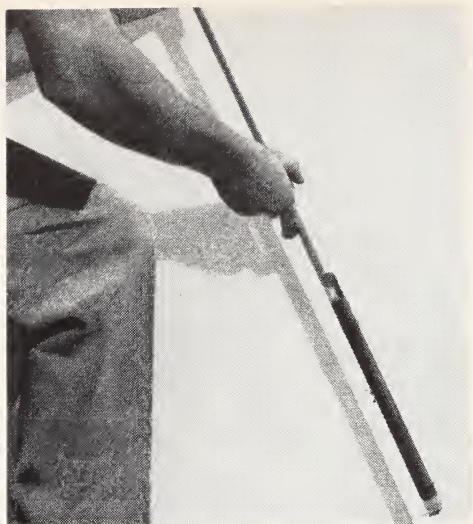
Fig. 19. Soil tube for checking field moisture.
