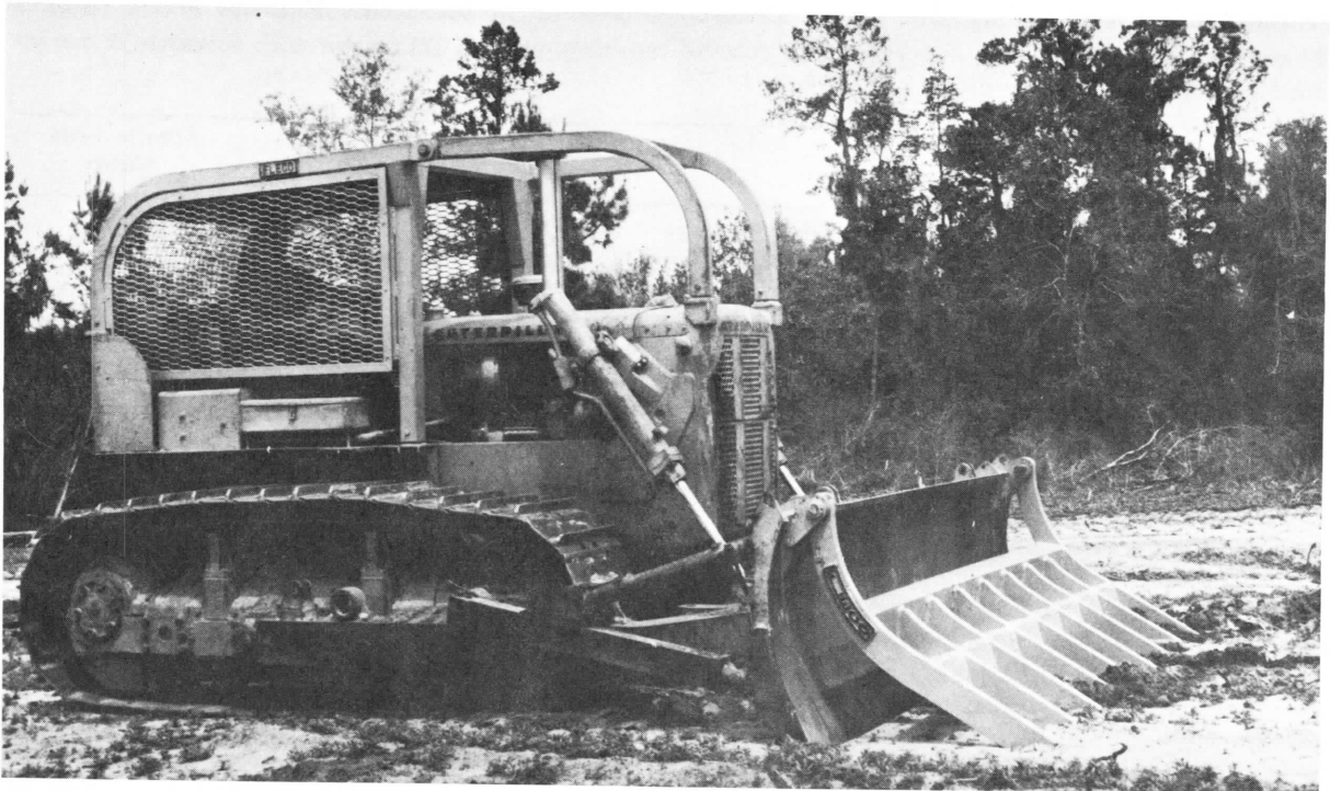
Fig. 2. Brush rake attachments generally are less effective than brush rakes, but they can be removed, permitting the straight dozer blade to be used for other work. Photo courtesy of Fleco Corporation.
