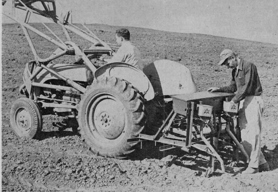
Equipment used for placement of seed and fertilizer in the Shasta County Agricultural Extension Service test plantings. Mr. Walter Spivey, farm advisor (standing by the seeder box), designed modifications which make the planter effective.
