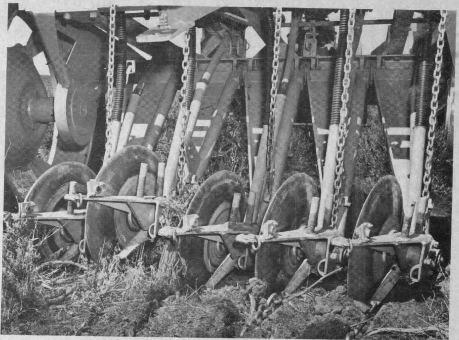
This is the type of heavy duty range drill used by Lawrence J. Fee, a Modoc County, Calif., cattleman interested in an easy way to rejuvenate his range.
