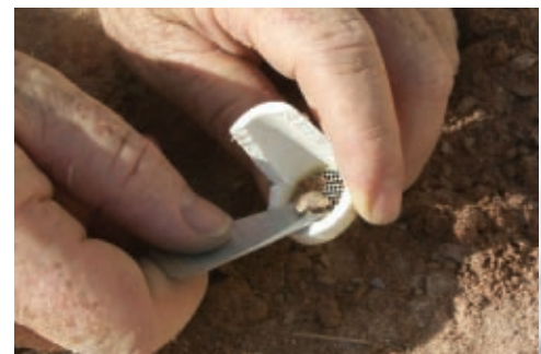
Figure 4. Place sample in sieve.
