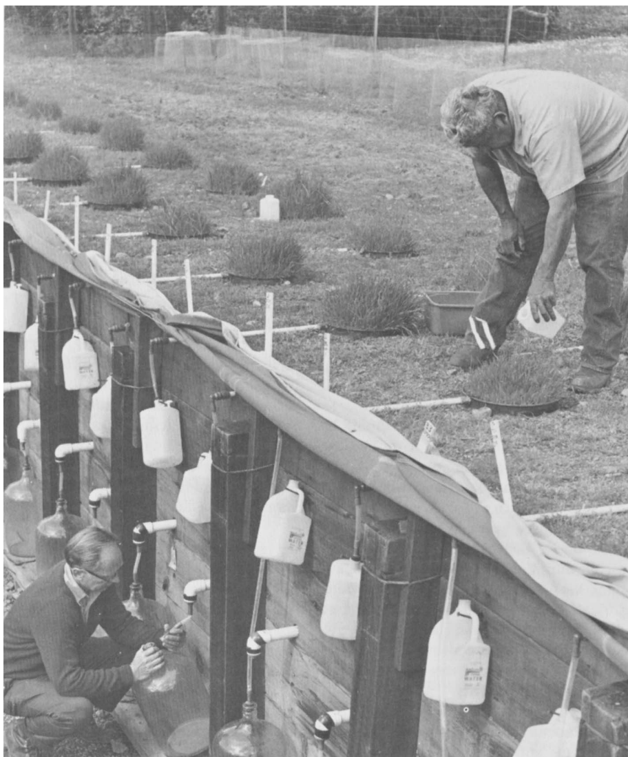
A lysimeter helps scientists determine loss of soil nutrients by leaching from different soil-plant combinations.
