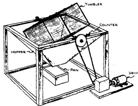
Specially built to approximate field raking to determine leaf shatter the tumbler—2' by 2' by 3'—was made of reinforced hardware cloth, mounted on a frame and equipped with a pan to catch the shattered leaves.
