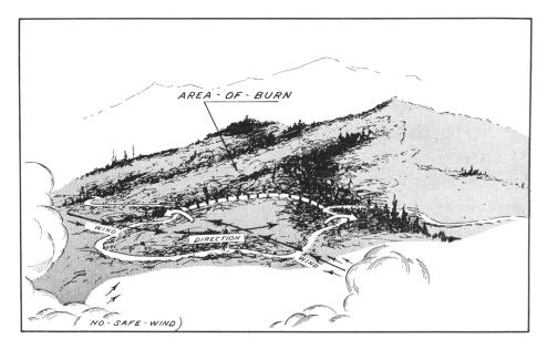
A road which follows the contour along the side of a hill often has U turns around ridges or in canyons. Here a shift in wind direction of a few degrees will blow fire over the road. A simple construction job, indicated by the broken line not only shortens the control line but the probability of slop-over and spot fires is greatly reduced, the work of firing and holding crews is minimized, and patrol is shortened.
