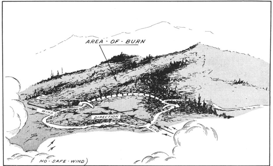
**A road which follows the contour along the side of a hill often has U turns around ridges or in canyons. Here a shift in wind direction of a few degrees will blow fire over the road. A simple construction job, indicated by the broken line not only shortens the control line but the probability of slop-over and spot fires is greatly reduced, the work of firing and holding crews is minimized, and patrol is shortened.**
