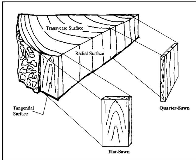
**Figure 2.** Structural Planes of Wood
