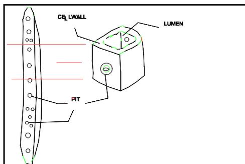
**Figure 4.** Sketch of a typical Softwood Tracheid
