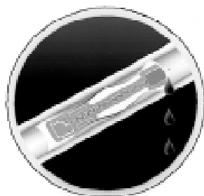
Figure 3. Cutaway example driptape emitter.
